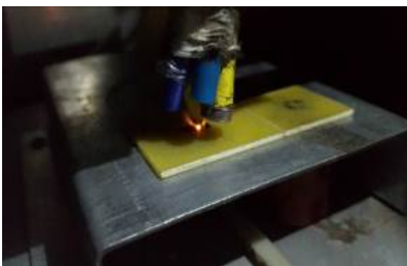
Figure 5: LASER vaporization of CNT-nickel composite
